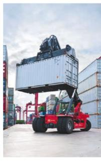
Intermodal Handling: toplift (twistlocks), trailer lift (lift legs) and slings (lift hooks).
