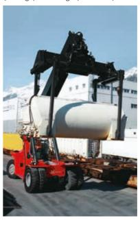
Industrial Handling: sub attachments (twistlocks) and slings (lift hooks).
