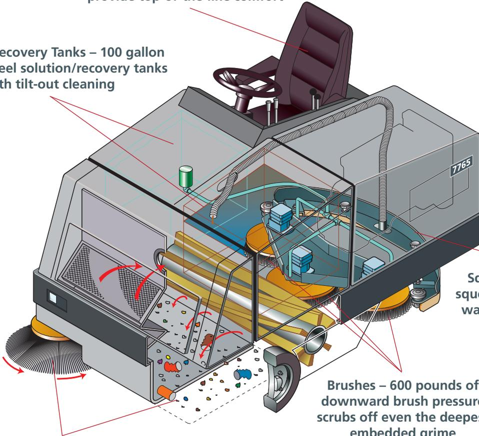
**Squeegee – Accu-Track™ squeegee provides superior water pickup even during the tightest turns**
